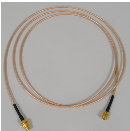
Figure 8: Wi-Fi antenna extension cable
