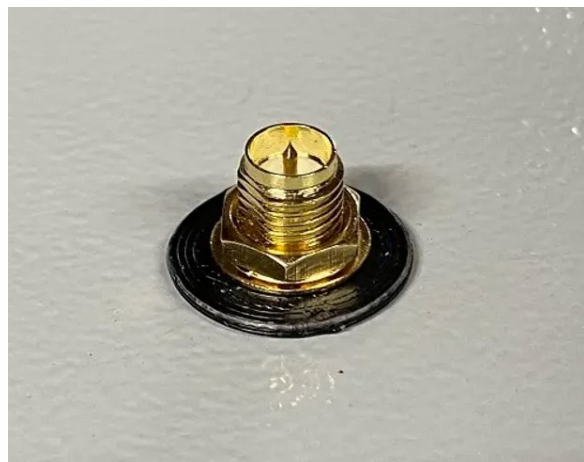
Figure 9: Antenna extension cable installed
